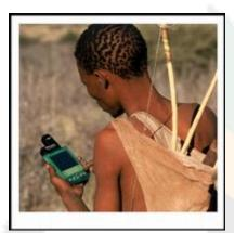
**The Cybertracker:** is a hand-held device that allows rangers to track animals in the field, by using the built-in GPS system and graphical interface. Because of the graphical interface, it is also possible for illiterate people to easily use this device. The Cybertracker, a modern **South African invention**, was the brainchild of Louis Liebenberg and Lindsay Stevenson.
